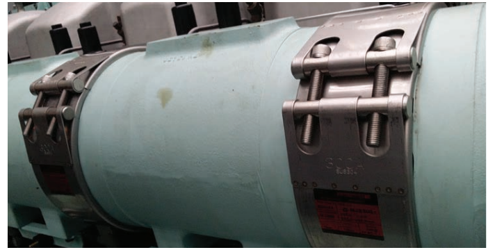
MJS NBR + strip insert 335mm, etc. medium speed propulsion engines & marine genset. Korea
