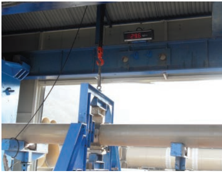
MJL 400A. pressure test on fiberglass pipe @29.6kg/cm 3 . Korea
